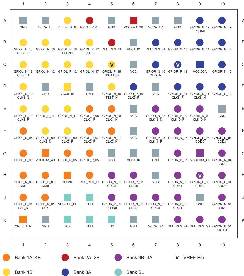
Figure 7: 100-Ball FBGA I/O Bank Diagram
