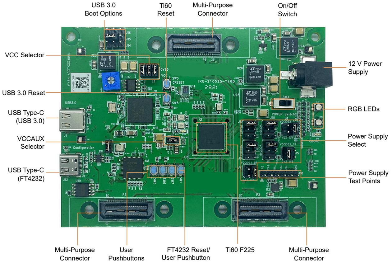
Figure 3: 钛金系列 Ti60 F225 Development Board Components (Bottom)
