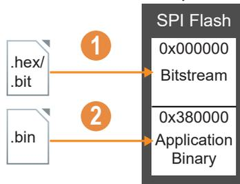
1. Program the board's SPI flash with the Ti60 example design bitstream.
