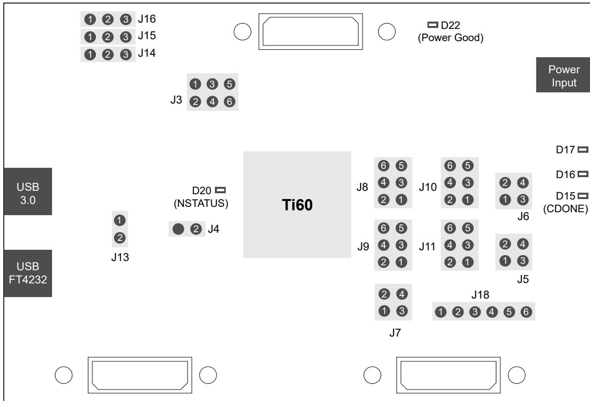
The 钛金系列 Ti60 F225 Development Board provides three multi-purpose 0.8 mm high-speed ground plane sockets. These sockets can be used for GPIO, MIPI CSI-2 TX/RX, and LVDS TX/RX. The board includes two USB type-C ports, one for USB 3.0 interface and the other for the FTDI interface.
