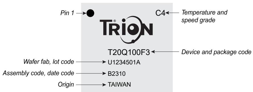
Figure 16: 100-Lead LQFP FPGA Package Outline
