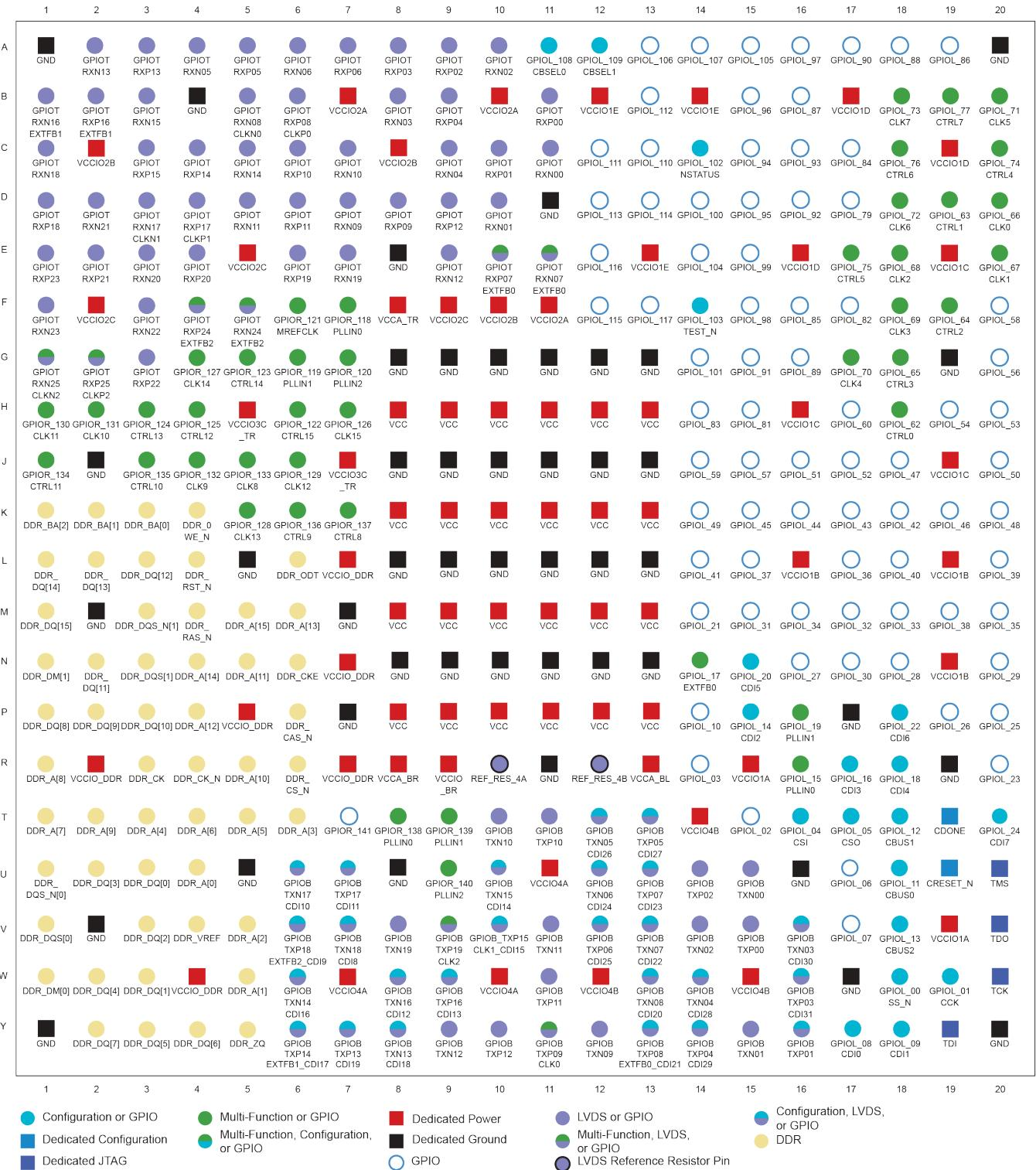
Figure 38: 400-Ball FBGA I/O Bank Diagram
