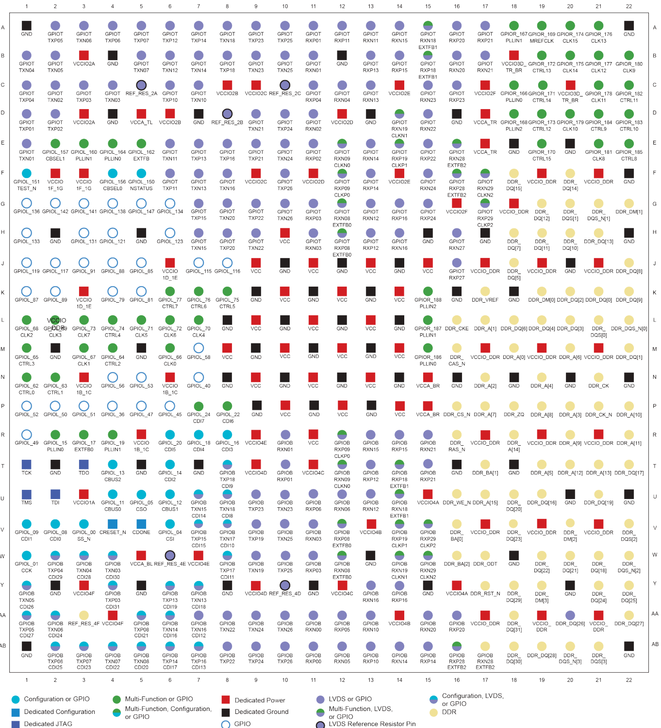
Figure 41: 484-Ball FBGA Pinout Diagram
